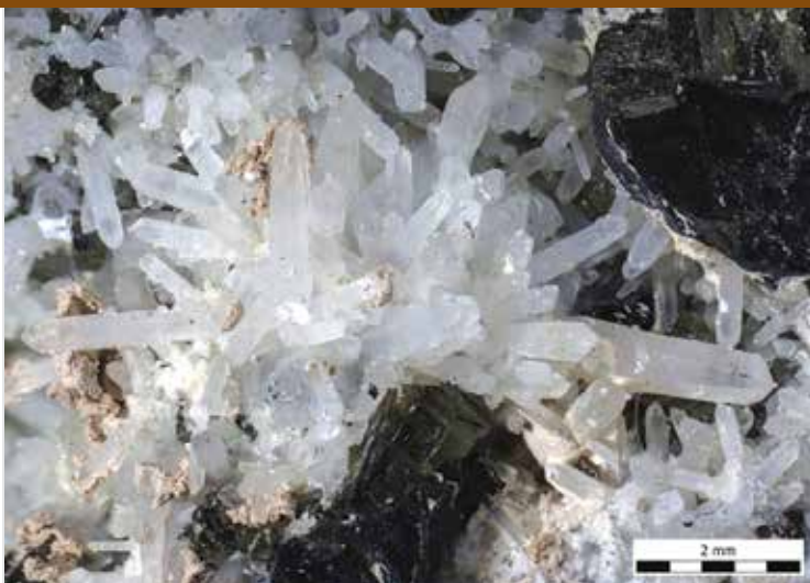
Drúza kremeňa analyzovaná stereomikroskopom SZ61-TR / Druse of crystal quartz analysed by stereomicroscope SZ61-TR
