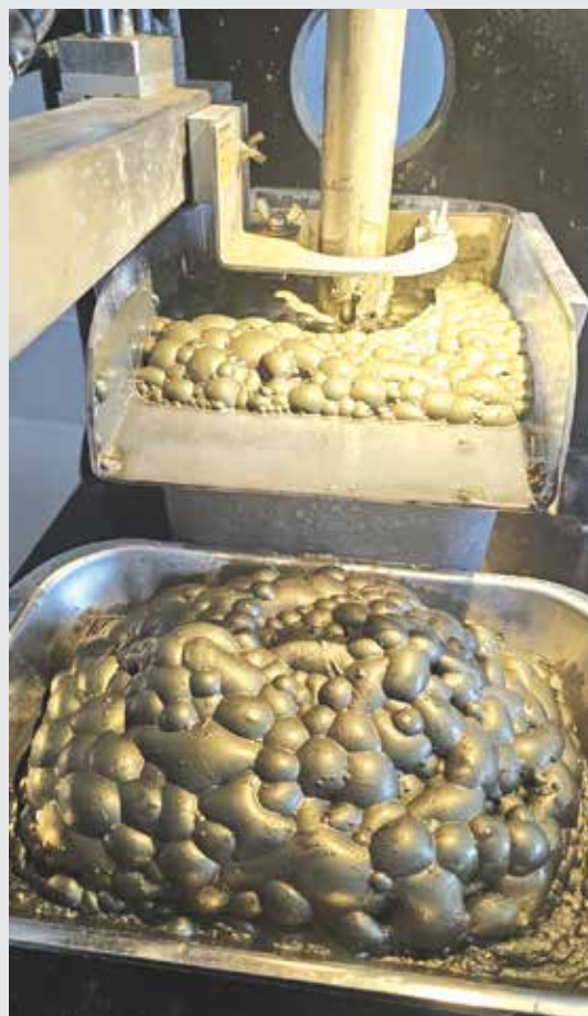
Laboratórna flotácia sulfidickej rudy / Laboratory flotation of sulphidic ore
