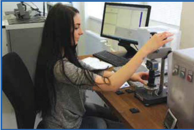
Meranie Shorevej tvrdosti gummy Determination the Shore hardness of rubber
