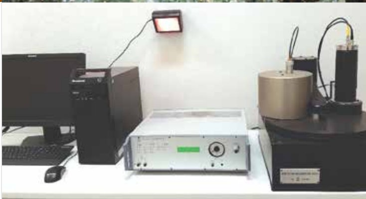
Datovacie zariadenie TL/OSL-DA-20 / Dating equipment TL/OSL-DA-20
