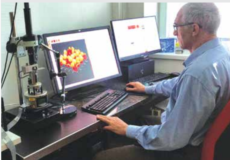
Mikroskop atomárnych síl (AFM) / Atomic force microscope (AFM)
