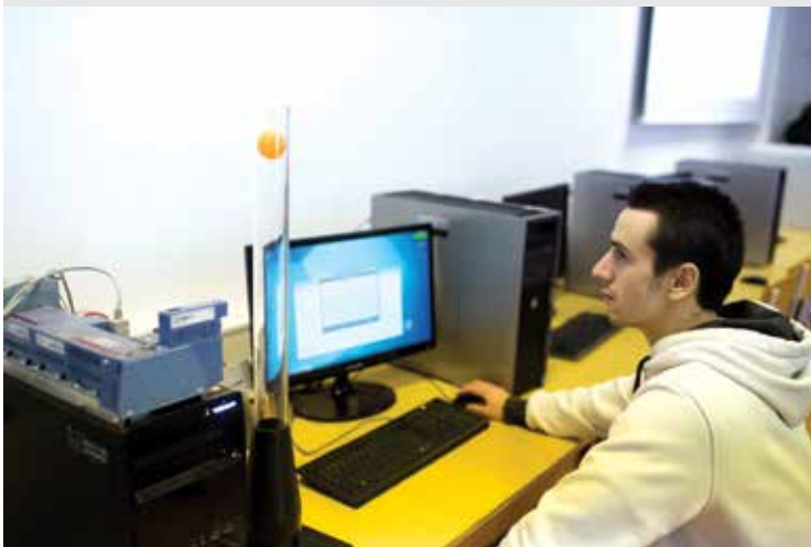
Ukážka riadenia polohy loptičky na PLC automate / Illustration of ball position control by PLC automata
