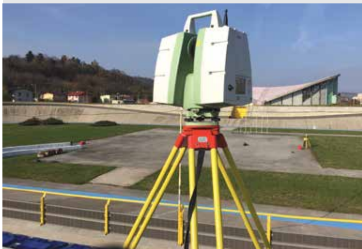
Leica ScanStation C10 a skenovanie velodromu v Prešove / Leica ScanStation C10 and velodrome scanning in Prešov
