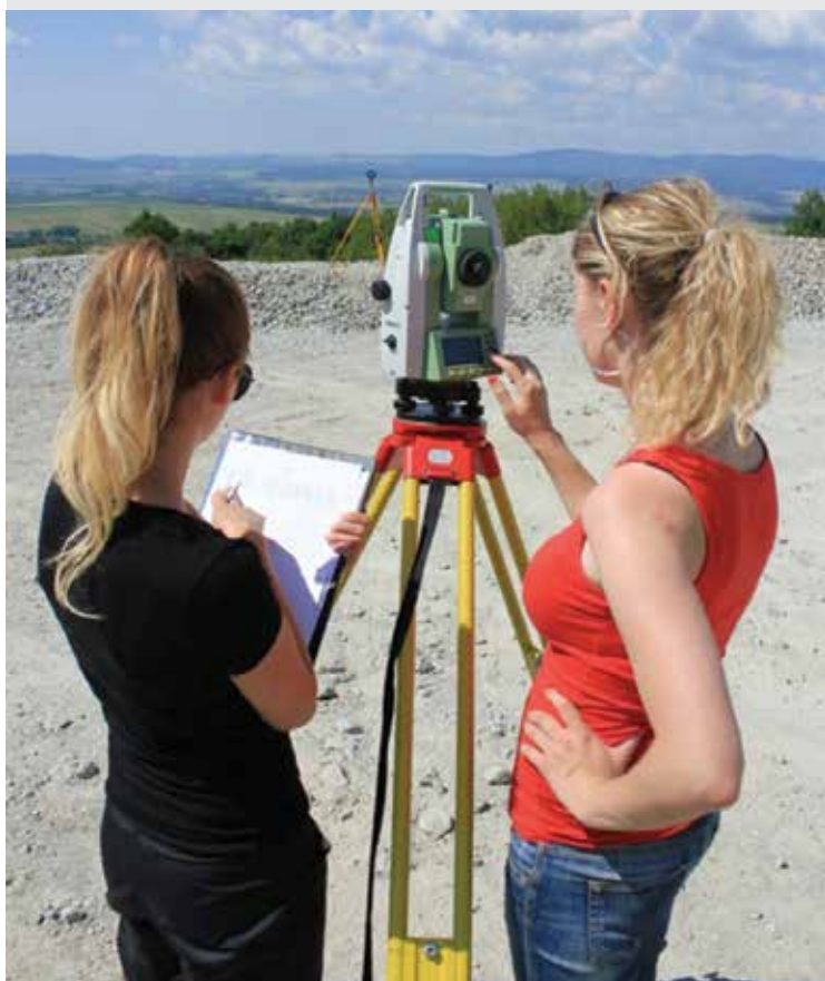
Terénne merania s UMS Leica TS06 / Field measurements with total station Leica TS06
